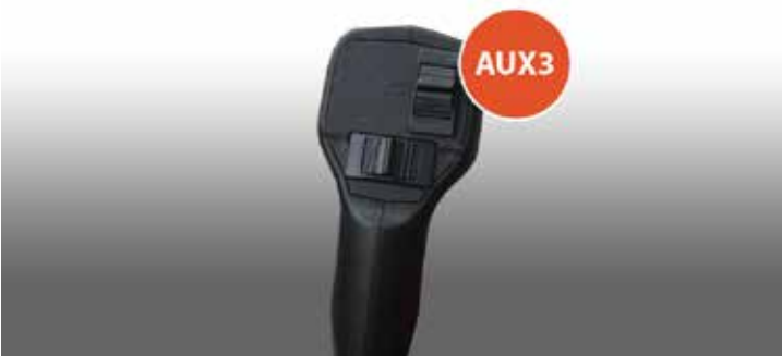
Proportional electronic roller for auxiliary hydraulic system on left Joystick (Tier3 models)
